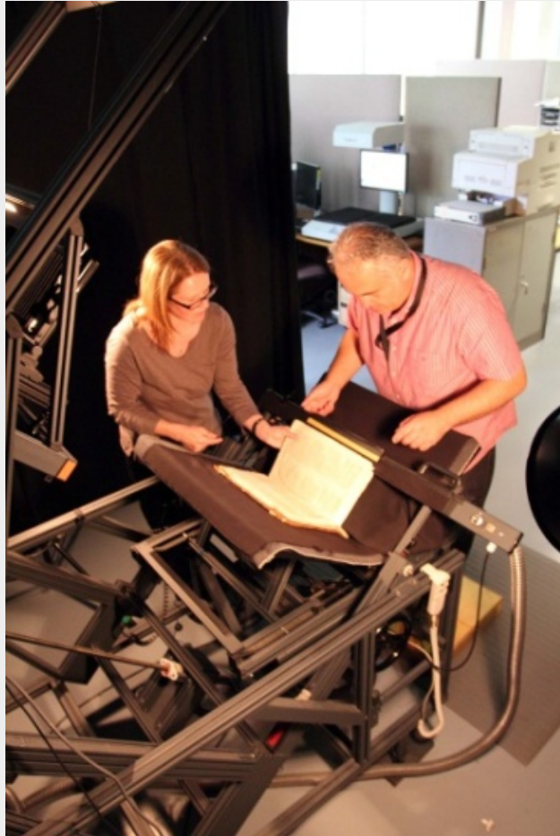
Conservator Nicole Gilroy and Photographer Nick Cistone digitising with Bodleian's Grazer Conservation Cradle in the Imaging Studio
