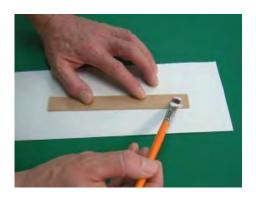
Before the adhesive on the spine dries, apply mixed adhesive to the single-thickness side of the tube.
