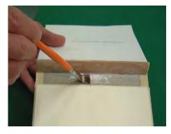
10. Before the adhesive on the tube dries, apply mixed adhesive to the lining of the cover spine.
