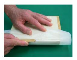
13. Use a folder to press the cover along the groove firmly into place.
