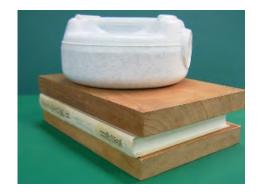
20. Place the book between two press boards, and place a weight on top of the upper board until the adhesive dries.
