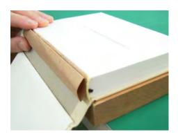
Attach the flattened tube to the face of the spine, taking care to align the tube to the spine.
