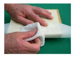
12. Cover the spine with cooking paper, then rub the spine and groove with a dry cloth to press the cover firmly in place on the text block.
