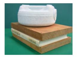
14. Place the book between two press boards, and place a weight on top of the upper board until the adhesive dries.
